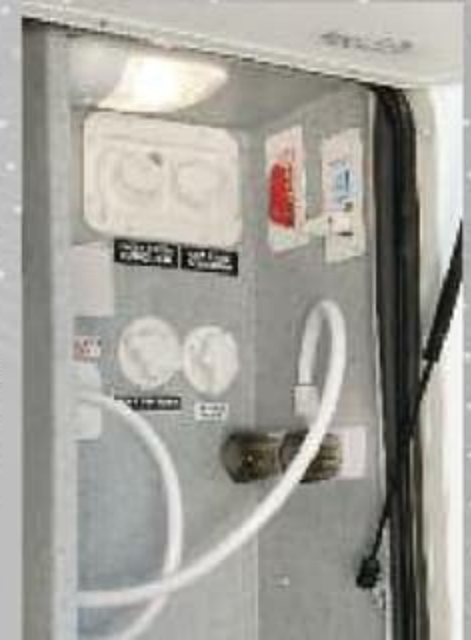
Exterior convenience center includes Within Reach water heater bypass valve, E-Z winterize valve, hot and cold exterior shower, black tank flush, 110V outlet plus cable and satellite hook-up
