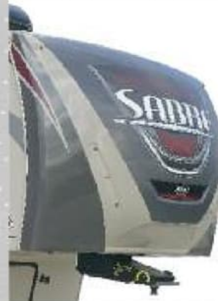
Aerodynamic fiberglass front cap with LED hitch pin and marker lights
