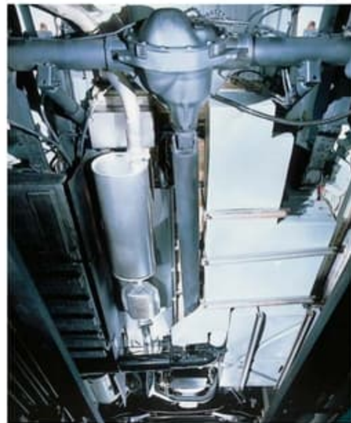
Water tanks fit below the floor which maximizes interior storage space. Locating them between the axles improves weight distribution for better handling.
