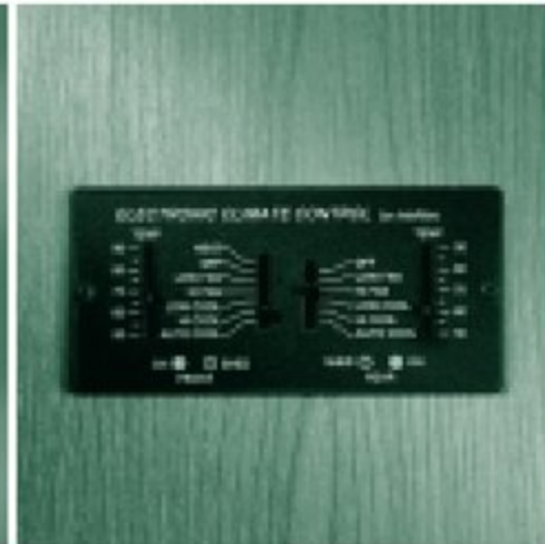
A standard electronic climate control system with dual A/C controls enables a separate climate in the front and rear of the coach.
