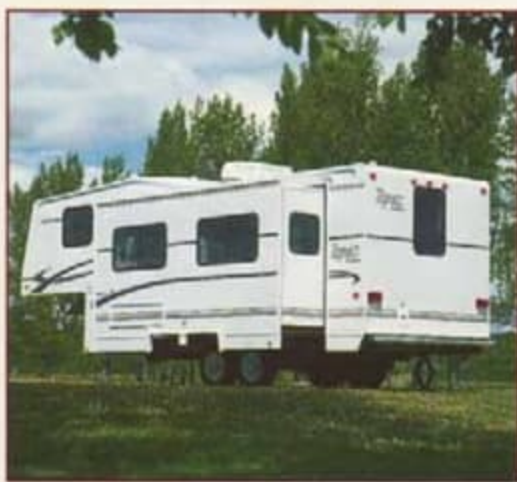
Radius corner slide windows are featured throughout the slide-out room.
