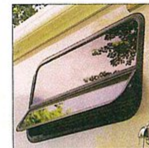
Windows feature tinted energy-saving "E-glass," and awning-style opening sections with screens. Window positions and sizes vary with floorplans.
