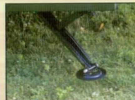
B.A.L. crank down jacks with sand pads are a standard feature on all Stampede and Thoroughbred travel trailers.
