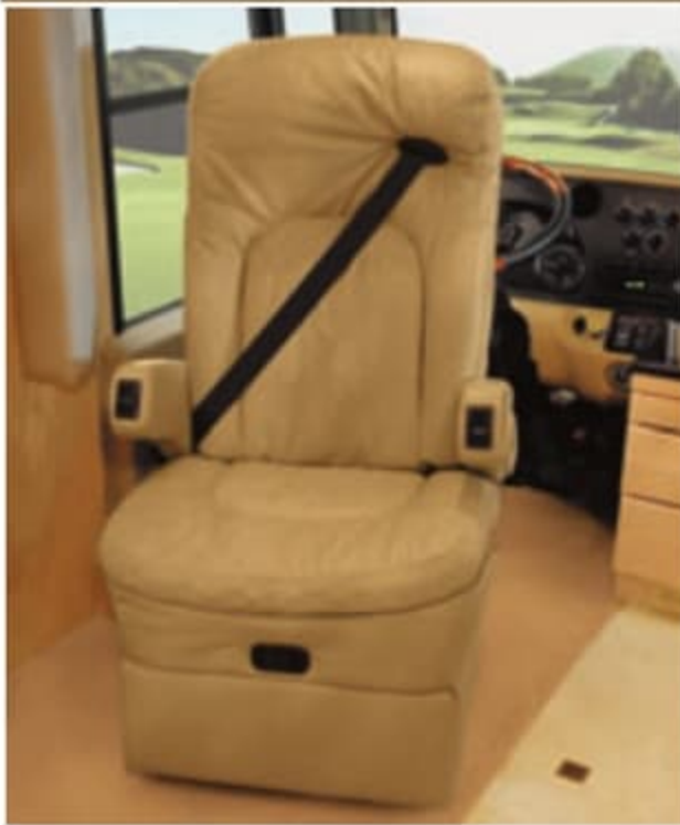
THE FLEXTSTEEL® LEATHER 8-WAY POWER DRIVER SEAT boasts 3-point integrated seat belts and heat and massage features for added comfort as well as lumbar support and memory settings to quickly adjust to each driver's preferences.
