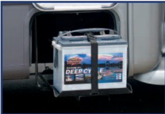
The slide-out battery tray provides quick and easy exterior access.
