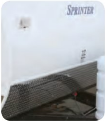
Sprinter diamond plate protects the front of the coach from road debris.
