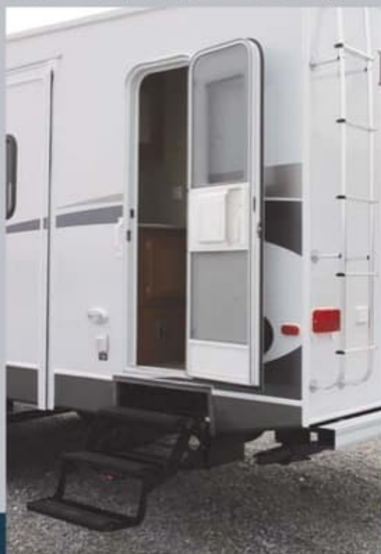
Rear entry door for optional second bath keeps sandy feet out of the living area (only available on 325BH)
