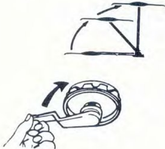
Raising the Antenna
