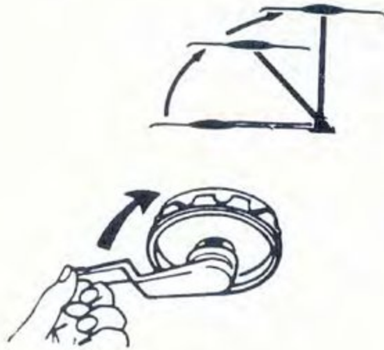
Raising the Antenna
