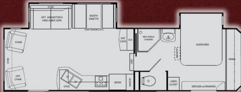
2800RLS GVWR: 11,380 lb. Length: 30'-10" Fresh: 57 gal. Dry: 7,975 lb. Height: 11'-10" Gray: 80 gal. Hitch: 1,875 lb. 12'-0" w/16" Wheels Opt. Black: 40 gal.
