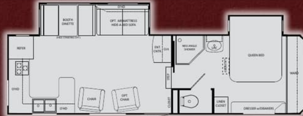
2900RK GVWR: 11,875 lb. Length: 31'-8" Fresh: 57 gal. Dry: 8,733 lb. Height: 11'-10" Gray: 80 gal. Hitch: 1,715 lb. 12'-0" w/16" Wheels Opt. Black: 40 gal.
