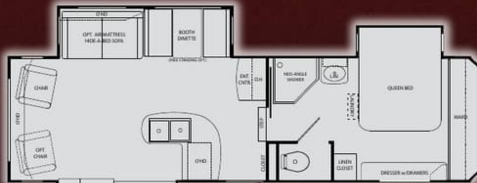
2900MK GVWR: 12,034 lb. Length: 31'-8" Fresh: 57 gal. Dry: 8,741 lb. Height: 11'-10" Gray: 80 gal. Hitch: 1,874 lb. 12'-0" w/16" Wheels Opt. Black: 40 gal.
