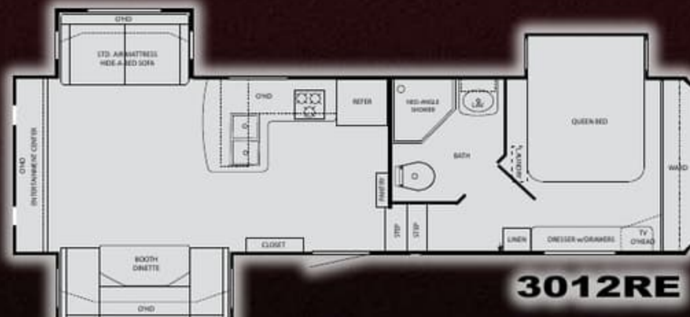
3012RE GVWR: 11,900 lb. Length: 32'-10" Fresh: 57 gal. Dry: 9,138 lb. Height: 11'-10" Gray: 80 gal. Hitch: 1,740 lb. 12'-0" w/16" Wheels Opt. Black: 40 gal.
