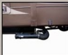
Rotating sewer boom provides more versatility when dumping the tanks
