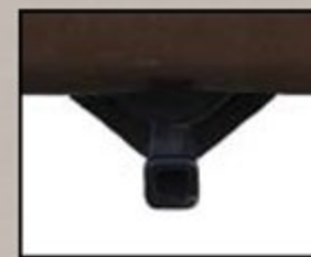
Receiver for a bike rack or utility cargo carrier (Up to 250 lbs)
