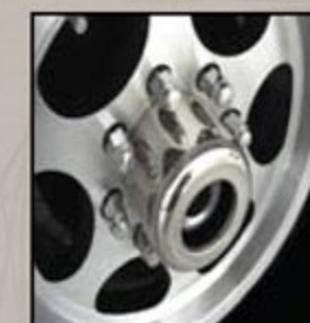
"Easy Lube" axles can be serviced without removing the wheel
