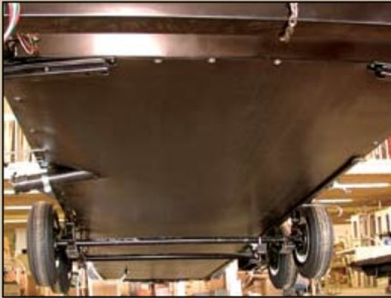
Outback's heated underbelly encloses tanks and valves, helping to extend the camping season.
