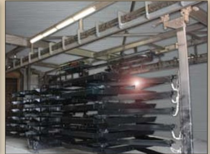
All Outback's are made with I-Beam chassis and full size outriggers that are powder coated and baked to ensure the most rust resistance available on the market.
