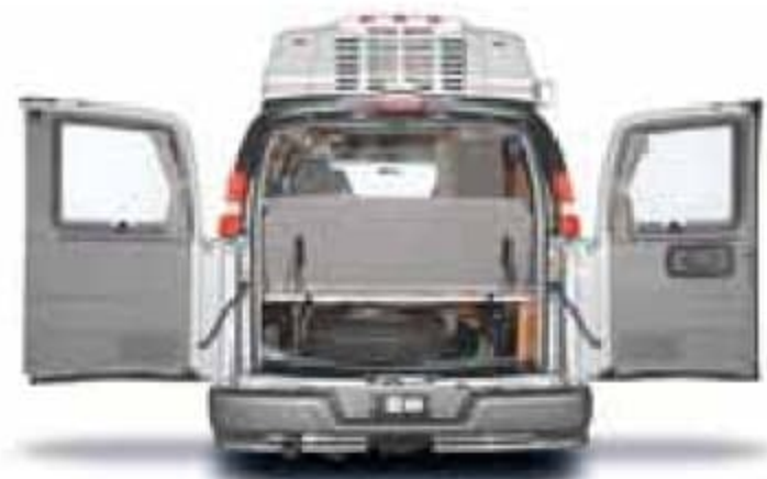
Dual rear doors allow for easy rear loading and swing a full 180° on 170 and 190 models and 270° on RS and SS models.
