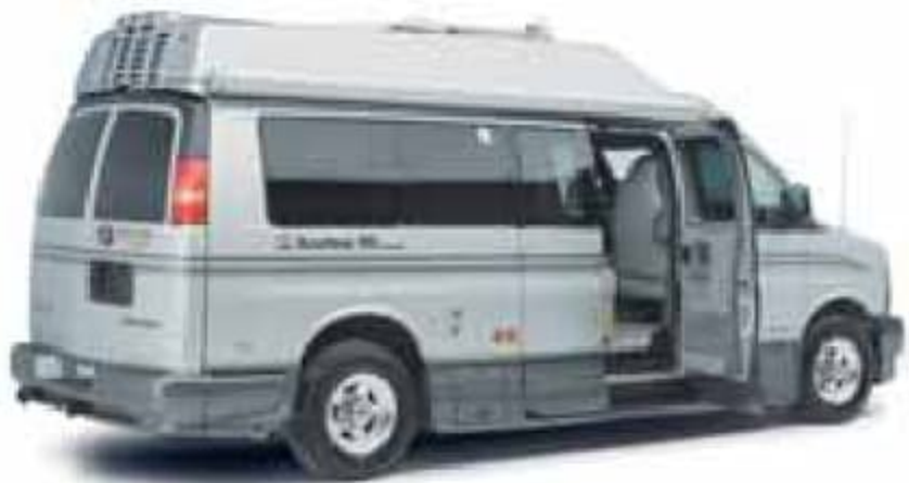
Easy entry is provided by a wide side door that features a low entrance floor and higher standing height. Large windows all around increase visibility.
