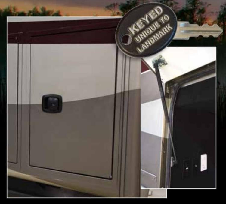
Enjoy the sleek, modern looks and functionality of LANDMARK's new optional bus style slam doors equipped with heavy duty struts for easy operation and they prevent unexpected closings due to wind. Oversized pull latches open easily. The tight automotive rubber seal protects your belongings from moisture and LANDMARK's compartments are keyed for security using keys and locks unique to LANDMARK.
