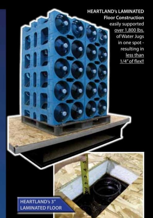
Heartland builds recreational vehicles with as many residential features and construction methods as possible and we are excited to introduce this 3" Laminated Floor System in our LANDMARK fifth wheels.
