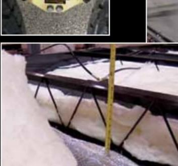
HEATED AND ENCLOSED UNDERBELLY This one-piece corrugated plastic underbelly is fitted and attached to the entire length of the fifth wheel, providing a thermal barrier that is easily removed for access to the underbelly. The underbelly area is insulated and heated from the furnace to help protect against the elements.
