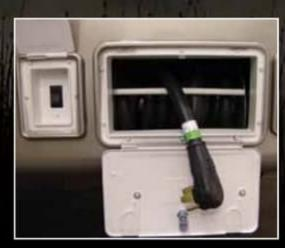
The electric power cord reel means you'll never have to wind that heavy 50-amp cord up by hand again!
