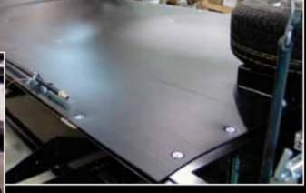
HEATED AND ENCLOSED UNDERBELLY This one-piece corrugated plastic underbelly is fitted and attached to the entire length of the fifth wheel, providing a thermal barrier that is easily removed for access to the underbelly. The underbelly area is insulated and heated from the furnace to help protect against the elements.
