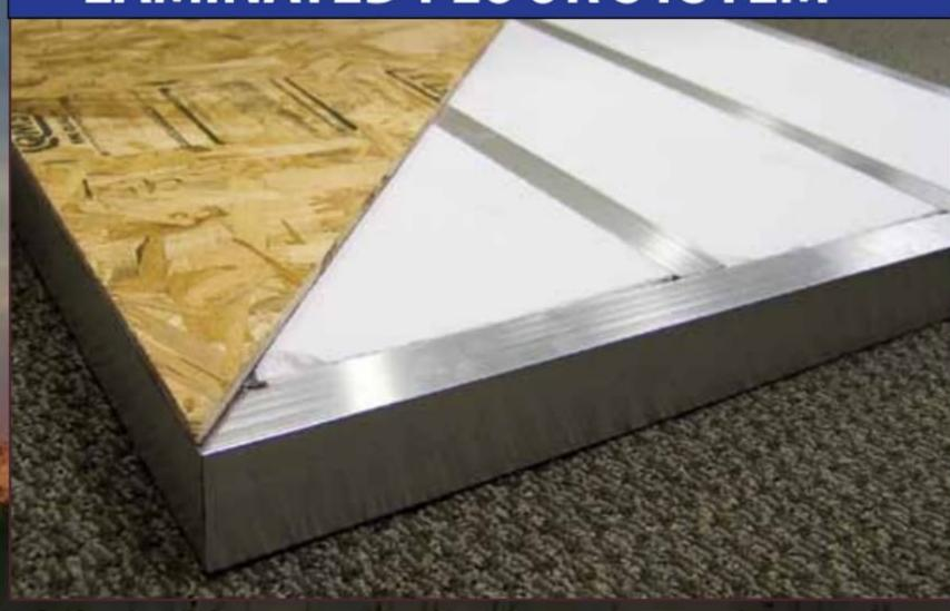
LANDMARK'S LAMINATED Floor System is one of the STRONGEST FLOORS in the industry! Featuring sturdy 2.5" Aluminum Framing; thick Block Foam Insulation; One-Piece Seamless Decking and a Thermo-Board Luan on the bottom. All of this is Laminated together for Maximum Strength and Insulation R Value - virtually eliminating flex in the floor!
