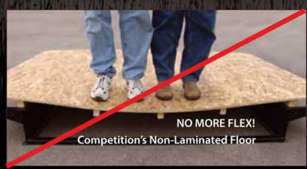
Traditional RV Floor Construction often flexes in the middle of the coach - because that's where the holding tanks are located and there is no steel frame support under the lumber.
