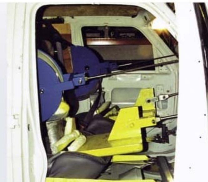
These 2 photos depict simultaneous seat belt pull testing and seating system testing. Seat belt testing confirms proper seat belt location and minimizes the possibility of anchorage failures. Seating system testing verifies the integrity of the seats, their attachments, mounting hardware and installation.
