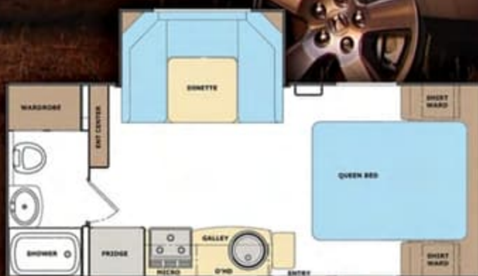
1985 18'10" INTERIOR FLOOR LENGTH 23'4" OVERALL EXTERIOR LENGTH 3670 POUNDS GROSS DRY WEIGHT
