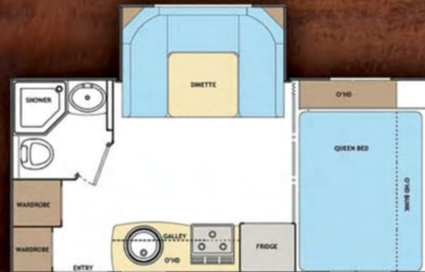
1685 16'3" INTERIOR FLOOR LENGTH 20'9" OVERALL EXTERIOR LENGTH 3450 POUNDS GROSS DRY WEIGHT
