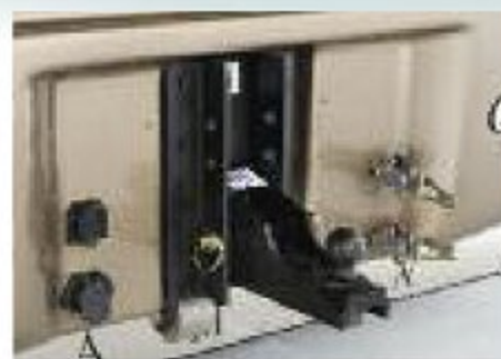
The optional 40,000 lb. rugged rear hitch helps provide you with twenty tons of towing power
