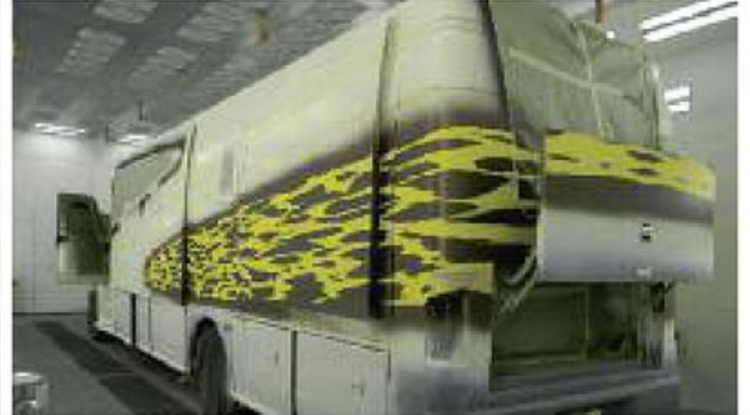
After masking to protect the previous coat, silver is applied
