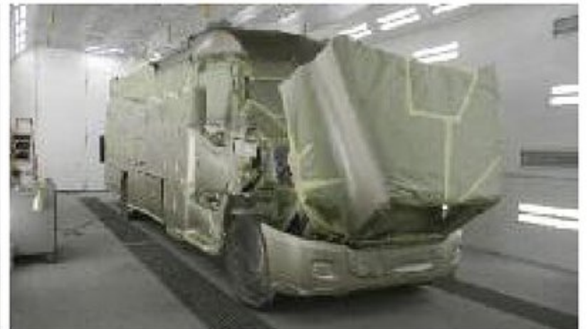
Final base coat color has been applied, unit will be unmasked to prepare for clear coat
