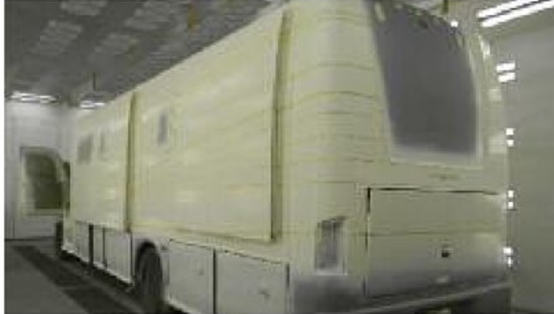
Digitally plotted, spray mask is carefully applied
