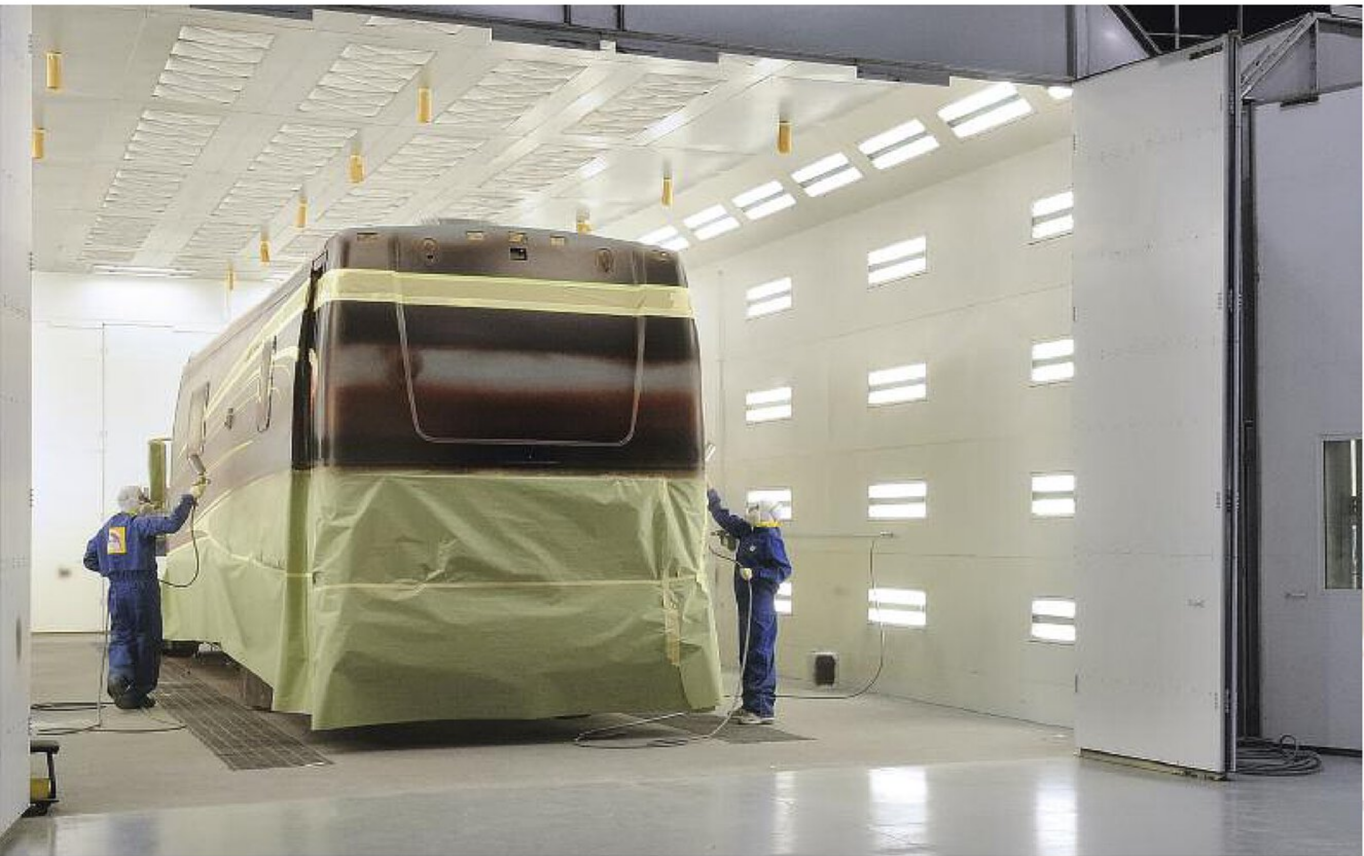
Legendary Five Step Paint - Three on-site 25' x 60' down draft bake booths can apply any custom paint scheme you can dream up.
