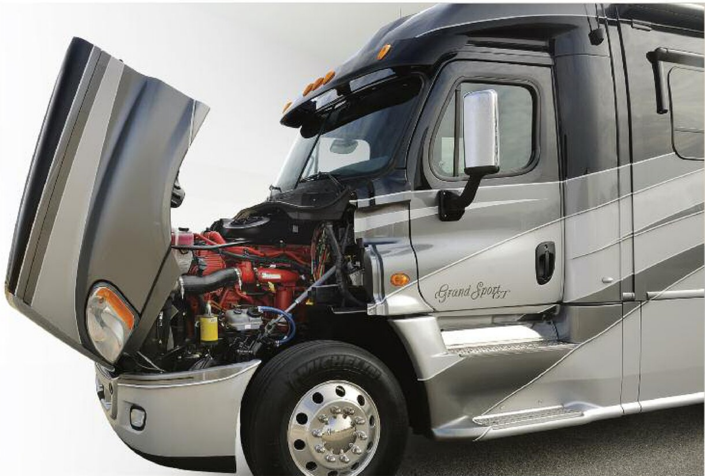
Easy Access All Grand Sport GT Models are built on the Freightliner Cascadia chassis and feature a flip front end to allow easy servicing of the engine compartment.
