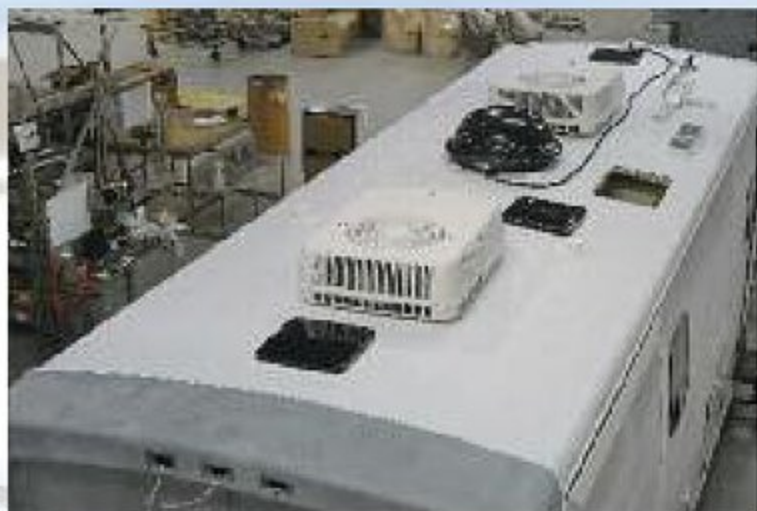
The F-Series is equipped with a one piece, radiused and laminated fiberglass roof.
