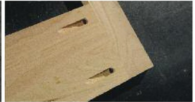
Pocket screws for structural integrity
