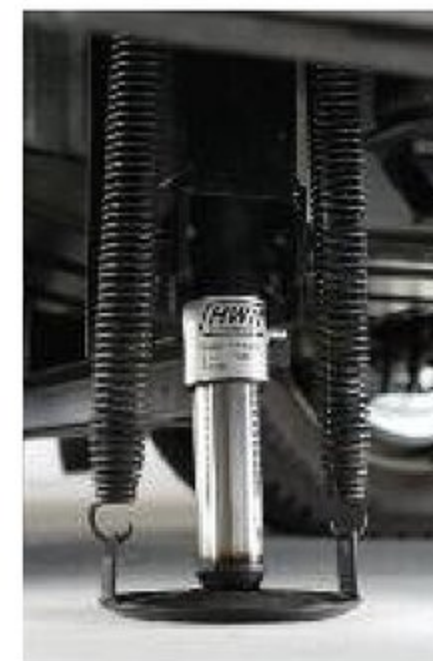
HWH CORPORATION The HWH fully automatic hydraulic four-point leveling system is standard on the F-Series.
