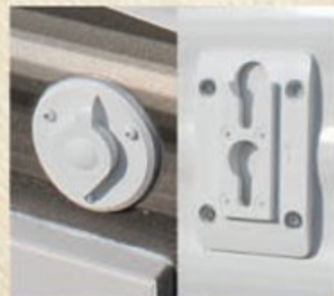
EXTERIOR TV HOOKUP/ CABLE AND BRACKET
