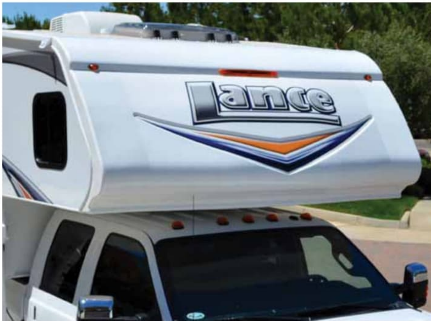
Aerodynamic Nose Cap for 2013 is made of TPO – the same material used for bumpers on automobiles. Its high gloss finish is resilient and resistant to the abuses of the road. And it's slick surface makes it easier to clean. (Selected Models)
