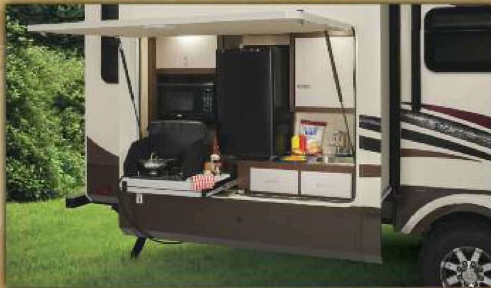
The 325RL's outdoor kitchen is equipped with weather resistant aluminum cabinets, drawers and countertop, plus a microwave, two-burner cooktop and refrigerator.
