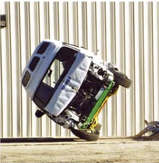
Dynamic rollover testing is intended to reduce deaths and injuries from occupants and their appendages not remaining within the passenger compartment during rollover accidents.
