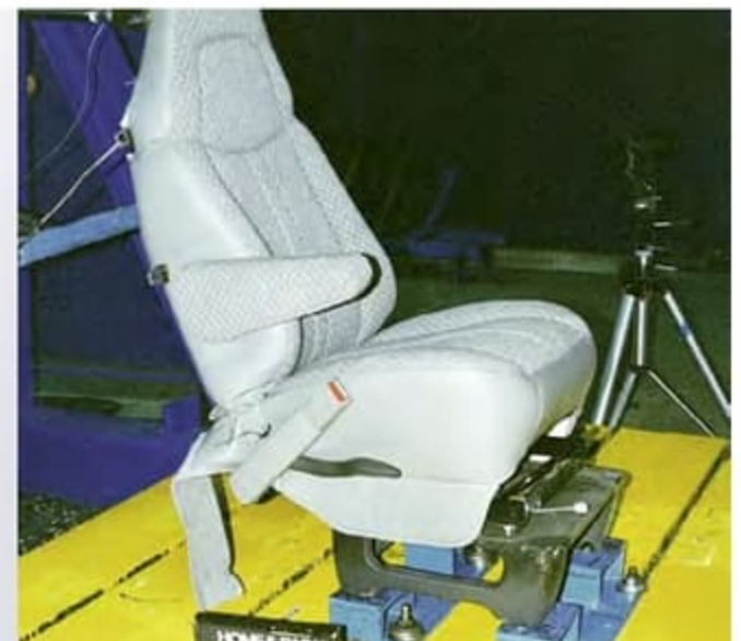
Seating system testing minimizes the possibility of failure of the seats, their attachments and their installation.
