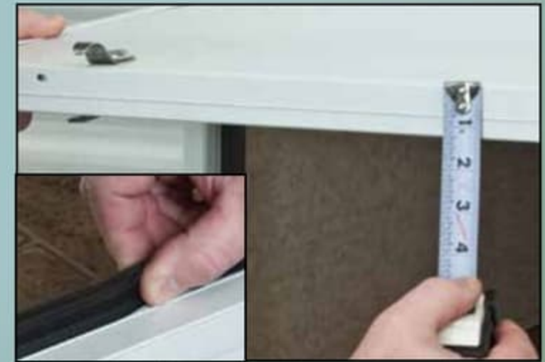
Thick insulated baggage doors with seamless aluminum door frame, no visible mounting screws and rubber seals protect your cargo.
