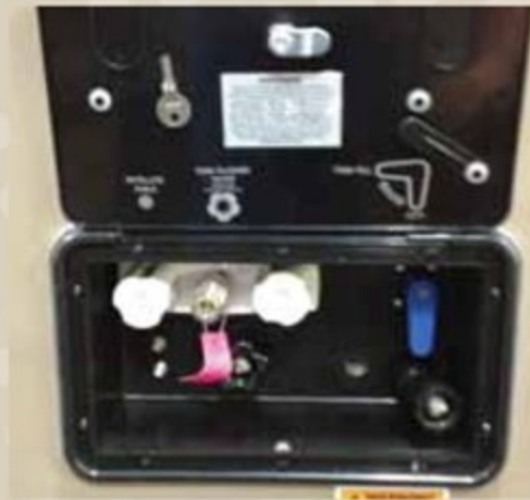
The X-Lite docking station provides a convenient location for many of your set-up needs.
