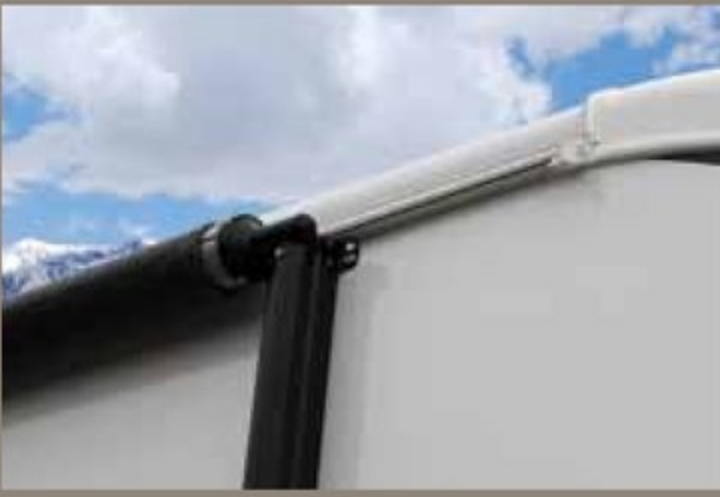
Rolled roof edge promotes increased water runoff
