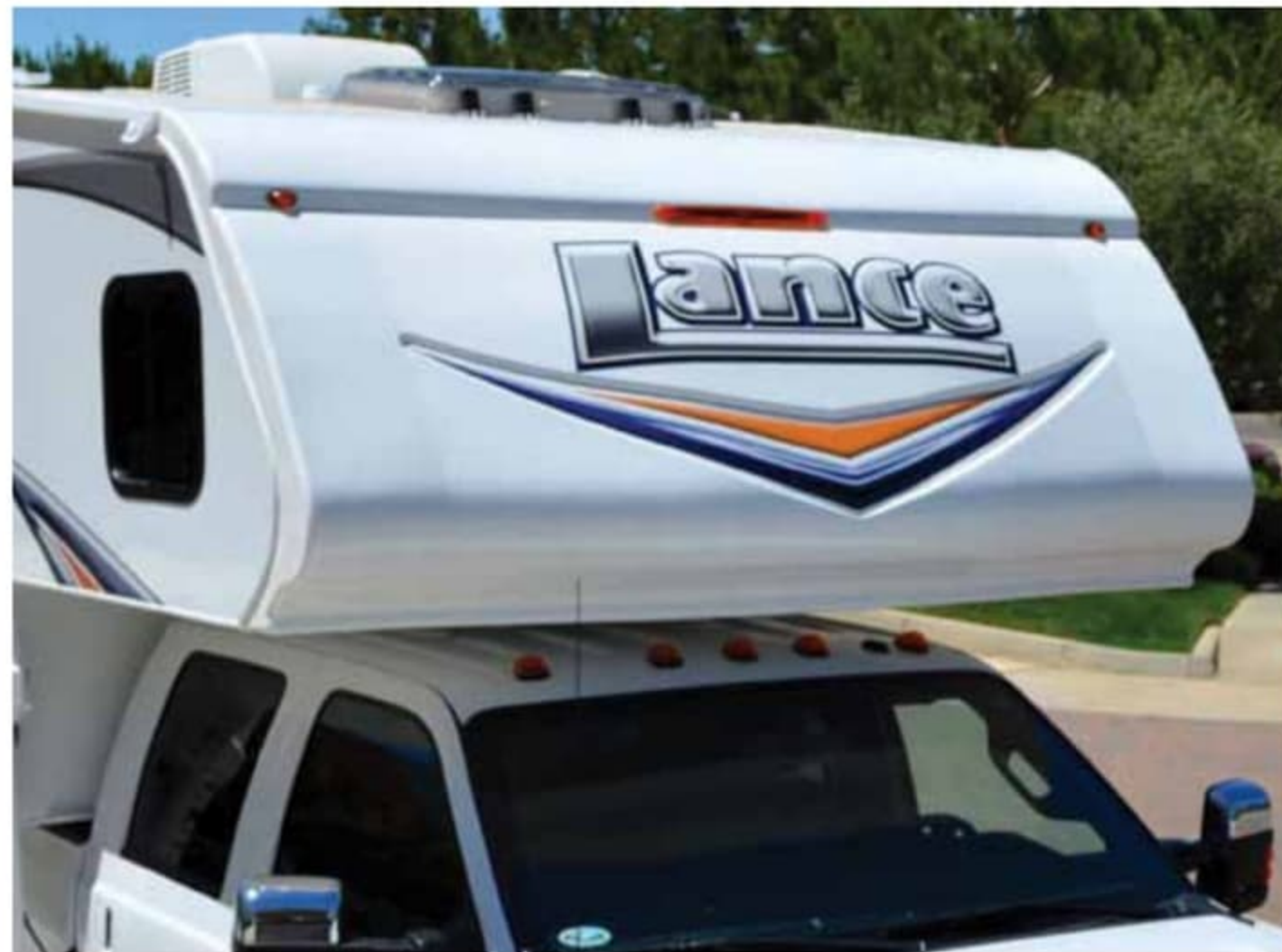
Aerodynamic Nose Cap is made of TPO – the same material used for bumpers on automobiles. Its high gloss finish is resilient and resistant to the abuses of the road. And it's slick surface makes it easier to clean (Select Models)
