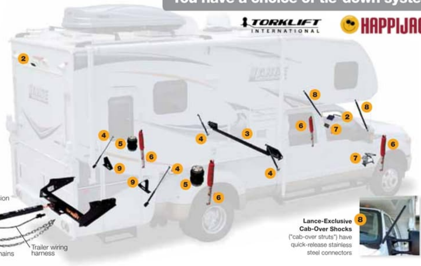
5 Within Air Lift's Super Duty Air Springs ("air bags") are the Lance internal jounce bumpers – which gradually cushion the suspension of the air springs as they approach the end of their jounce travel
