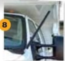
8 Lance-Exclusive Cab-Over Shocks ("cab-over struts") have quick-release stainless steel connectors
