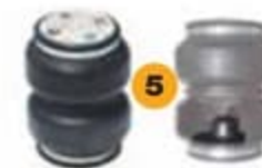
5 Within Air Lift's Super Duty Air Springs ("air bags") are the Lance internal jounce bumpers – which gradually cushion the suspension of the air springs as they approach the end of their jounce travel
