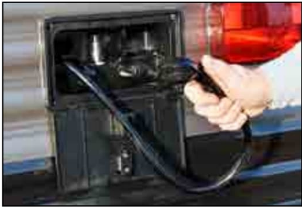
Outside Shower with hot and cold water.
