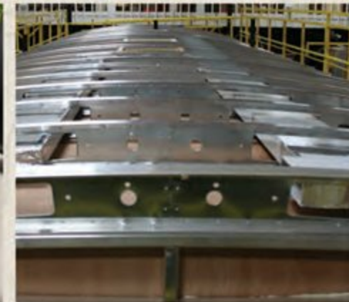
Walkable steel truss roof system
