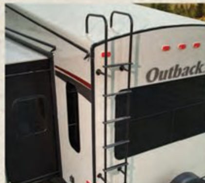
Rear roof ladder
