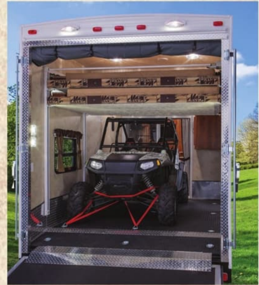
Garages include heavy duty D-ring tie-downs, anchored into an 8"x14" steel plate welded to the frame for secure travel. Dovetail diamond plate for safe, easy access.
