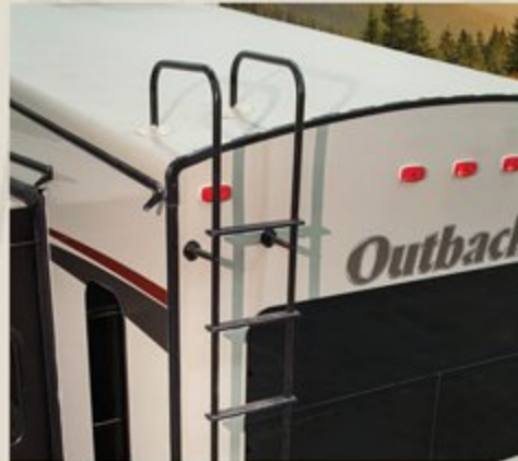
Rear roof ladder
