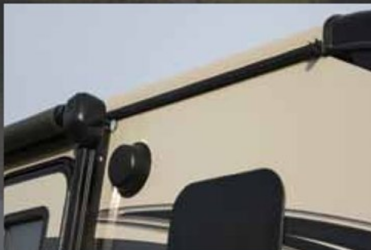
ROLLED ROOF EDGE PROMOTES INCREASED WATER RUNOFF
