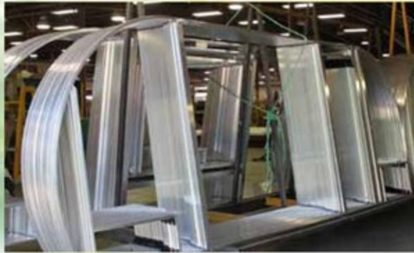
Winnie Drop features aluminum framing laminated with block foam insulation, true gel coat fiberglass exterior, and designer interior décor panels.
