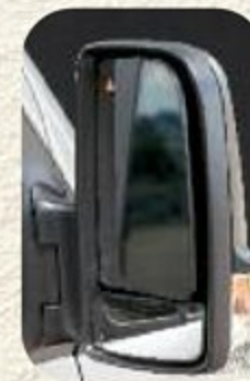
Chassis safety upgrades include a blind spot triangle on the side view mirror
