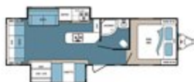
DENALI TRAVEL TRAILER | 2975RL Ext. Length: 33' 9" Ext. Height: 11' 7" Average Shipping Weight: 7,250 Sleeps: 3-4
