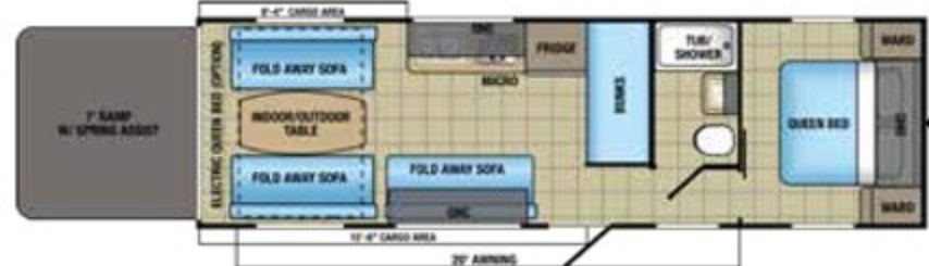
OCTANE SUPER LITE | 272 OPTIONS: A, B Ext. Lgth: 33' 11" Ext. Ht: 144" Unloaded Wt (lbs.): 7,050 Sleeps: 8-9
