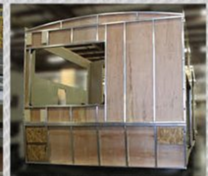
Double welded aluminum cage construction in walls and floors.
