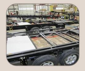
Competitors install a one piece underbelly design which is screwed into the frame.
