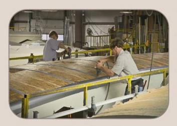
A full length 3/8" wood decking, for a full walk-on roof, is screwed, not stapled, into place. Our final step is adding a two-ply, Tuff ply™, rubber roof membrane with a built-in fire retardant and 12 year warranty.
