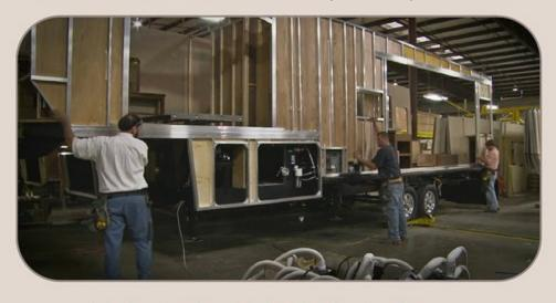
Individually fastened, custom "L" brackets combined with 3M Silaprene adhesives are designed to bend, flex and absorb road stress. 3M® Silaprene adhesives have a 475 PSI (Pounds per Square Inch) and get stronger as it ages. It is resilient and has outstanding resistance to moisture, road chemicals, heat, and cold.
