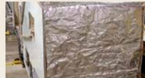
R-38 Radiant shield Thermo-foil wrap through ceilings, underbellies and under front caps.
