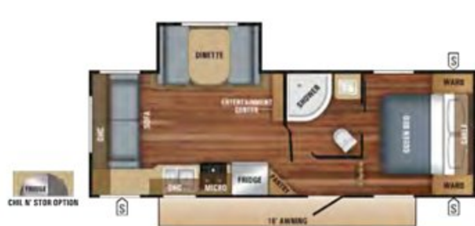
JAY FLIGHT SLX | 245RLS OPTION A Ext. Lgth: 28' 2" Ext. Ht: 132" Unloaded Wt. (lbs): 5,220 Sleeps: 4-6
