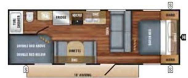
JAY FLIGHT SLX | 264BH Ext. Lgth: 29' 3" Ext. Ht: 126" Unloaded Wt. (lbs): 4,615 Sleeps: 8-10
