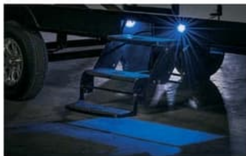
Safety step is triple step with built-in blue LED safety light.
