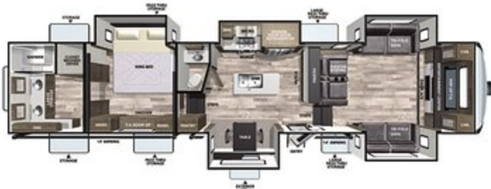
370FLX FRONT LIVING, RAISED BEDROOM, DUAL VANITY BATH, & 1/2 BATH WEIGHT: 14,414 LB. LENGTH: 41' 2"
