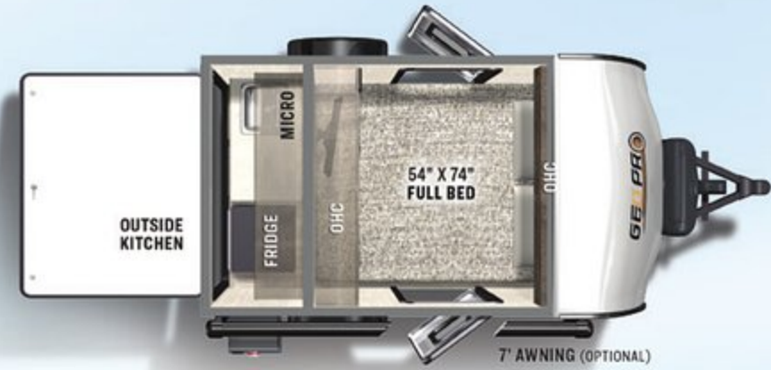
12RK REAR KITCHEN U/VW: 1252 HITCH: 162 AXLE: 1052 CCC: 710 LENGTH: 11'3" WIDTH: 6'8" GEO PRO HEIGHT: 7'9" INT. HEIGHT: 4'10" FRESH: 20 gal GRAY: 6 gal BLACK: NA
