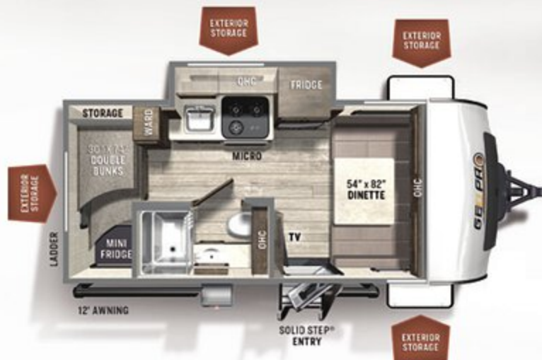
16BH BUNKHOUSE U/VW: 3200 HITCH: 461 AXLE: 2701 CCC: 761 LENGTH: 18'6" WIDTH: 7'8" GEO PRO HEIGHT: 9'10" INT. HEIGHT: 6'6" FRESH: 31 gal GRAY: 30 gal BLACK: 30 gal
