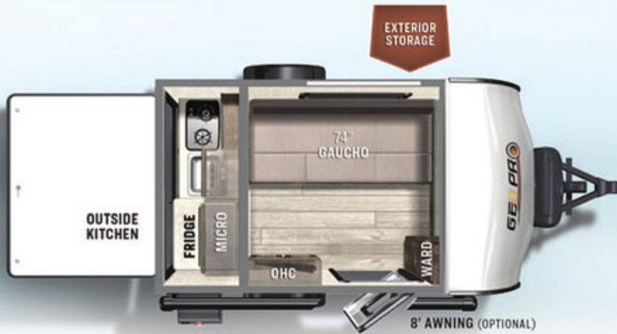
12SRK REAR KITCHEN U/VW: 1763 HITCH: 258 AXLE: 1467 CCC: 1135 LENGTH: 12'3" WIDTH: 7'4" GEO PRO HEIGHT: 7'9" INT. HEIGHT: 4'10" FRESH: 20 gal GRAY: 6 gal BLACK: NA
