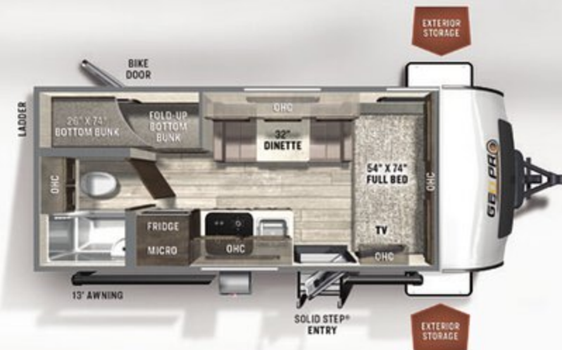
19BH BUNKHOUSE U/VW: 3178 HITCH: 411 AXLE: 2729 CCC: 1133 LENGTH: 20'2" WIDTH: 7'8" GEO PRO HEIGHT: 9'10" INT. HEIGHT: 6'6" FRESH: 31 gal GRAY: 30 gal BLACK: 30 gal
