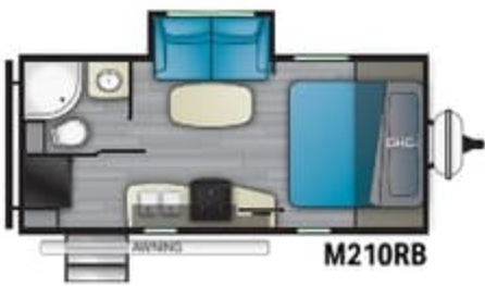
M210RB Length - 22' 1" Dry - 4,598 lbs. Hitch - 550 lbs. Height - 11' 4" GVWR - 6,900 lbs.
