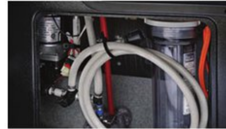
Winterizing tube provides easy access for quick maintenance includes bypass valve. (N/A 2250SLE, 2550DSLE)
