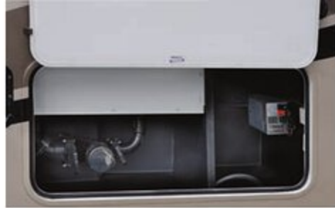
Heated/enclosed holding tanks use warm air from the furnace to protect tanks and valves. (N/A 2250SLE, 2550DSLE, MBS and Transit)
