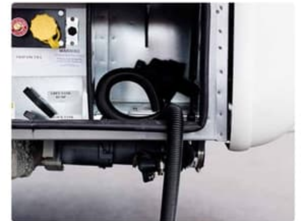
Macerator Sewage Discharge With Manual Disconnect
