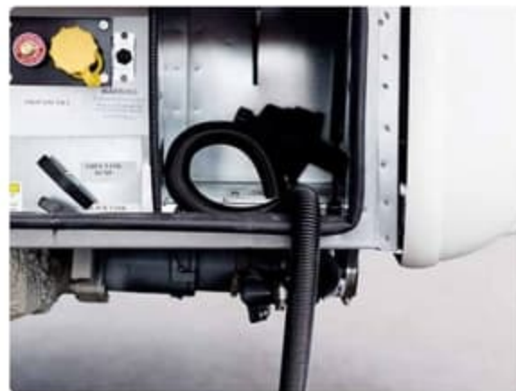
Macerator Sewage Discharge With Manual Disconnect
