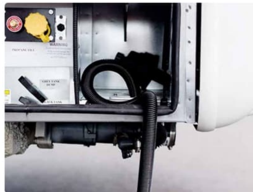
Macerator Sewage Discharge With Manual Disconnect
