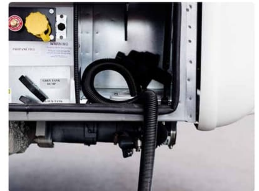
Macerator Sewage Discharge With Manual Disconnect
