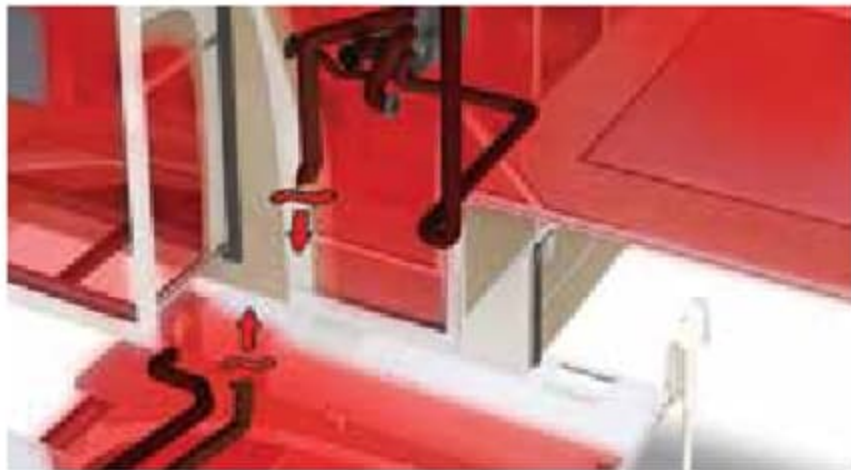
Ducted heat is routed into individually insulated holding tanks to keep them, the valves and PEX lines warm.
