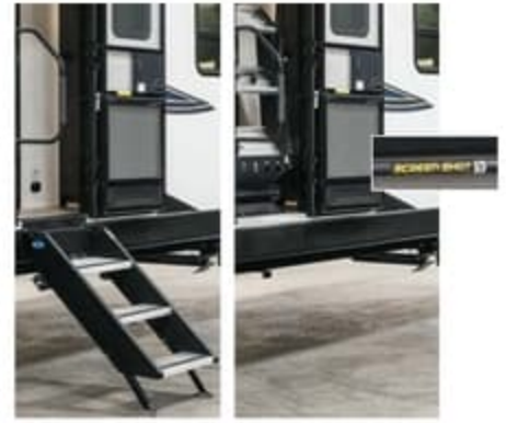
All SportTreds feature a solid flip-up step and friction-hinged entry door with Screen Shot screen door.
